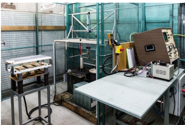
Partial Discharge Testing
